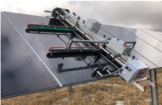
Figure 1: Cleaning Robot in operation
